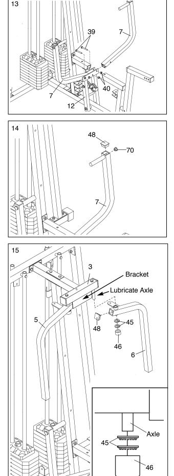
Press a 1 3/4" Square Inner Cap (48) into the lower end of the Left Arm (6). Wet the lower end of the Left Arm with soapy water. Slide a 10" Pad (45) onto the Left Arm.
